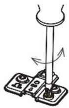
Height adjustment +/- 2mm
