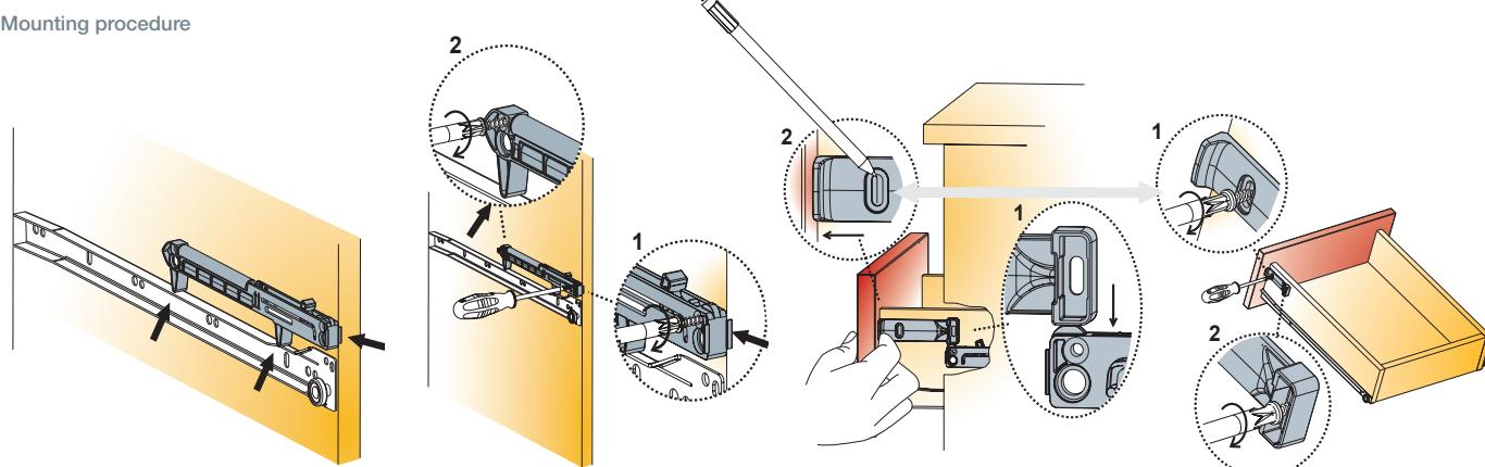
Position the Titusoft housing with the posts resting on the top of the drawer slide and the front tab touching the cabinet side
