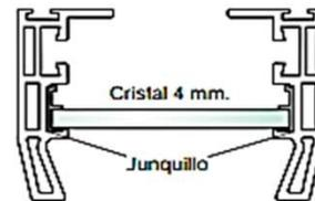
**KIT PERFIL HORIZONTAL SUPERIOR E INFERIOR COPLANAR M35 Y M50**
